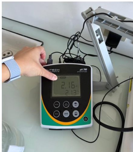
The pH determination of 0,1M NaOH solution and adjusting it to pH 2,16
